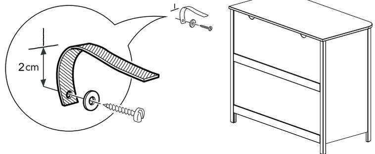
ENG: Using the wood screw and washer supplied, attach fixing strap to the underside of top panel.
