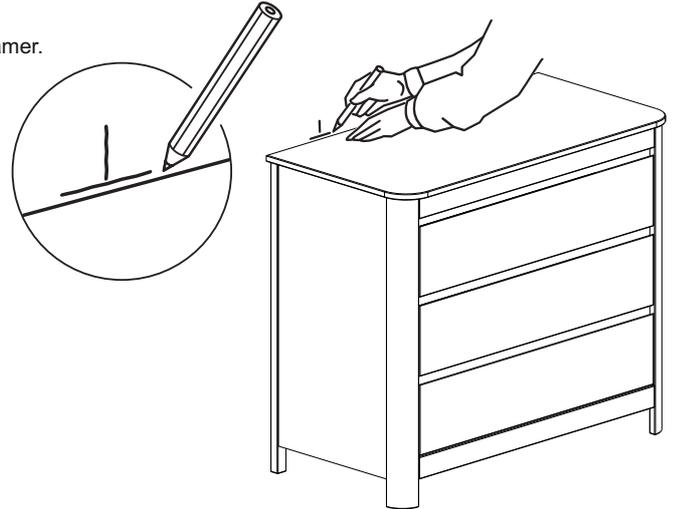
ENG: Attach fixing strap supplied to position on wall as shown. Ensure correct screws and fittings as appropriate to the type of wall are used. Check the wall is suitable for attaching this furniture.
