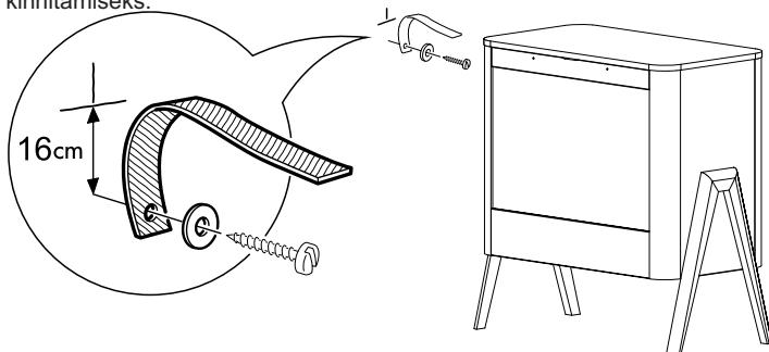
**ENG:** Using the wood screw and washer supplied, attach fixing strap to the underside of top panel,
