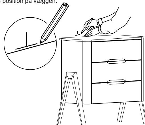
**ENG:** Attach fixing strap supplied to position on wall as shown. Ensure correct screws and fittings as appropriate to the type of wall are used. Check the wall is suitable for attaching this furniture.
